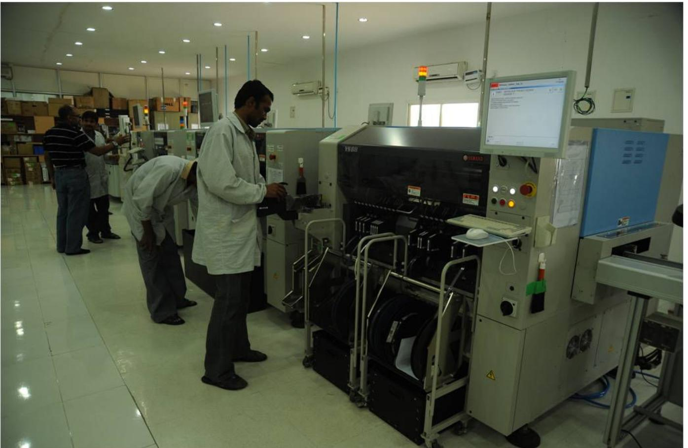
Description: Automated Pick & Place Component Insertion Line for Using SMT at VMC's Manufacturing Facility at Maheshwaram (Hyderabad)
